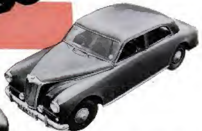
ALVIS Grey Lady, left, is a 100-mile-per-hour sedan with a high-compression, overhead-valve "square" engine and a seven-bearing crankshaft
